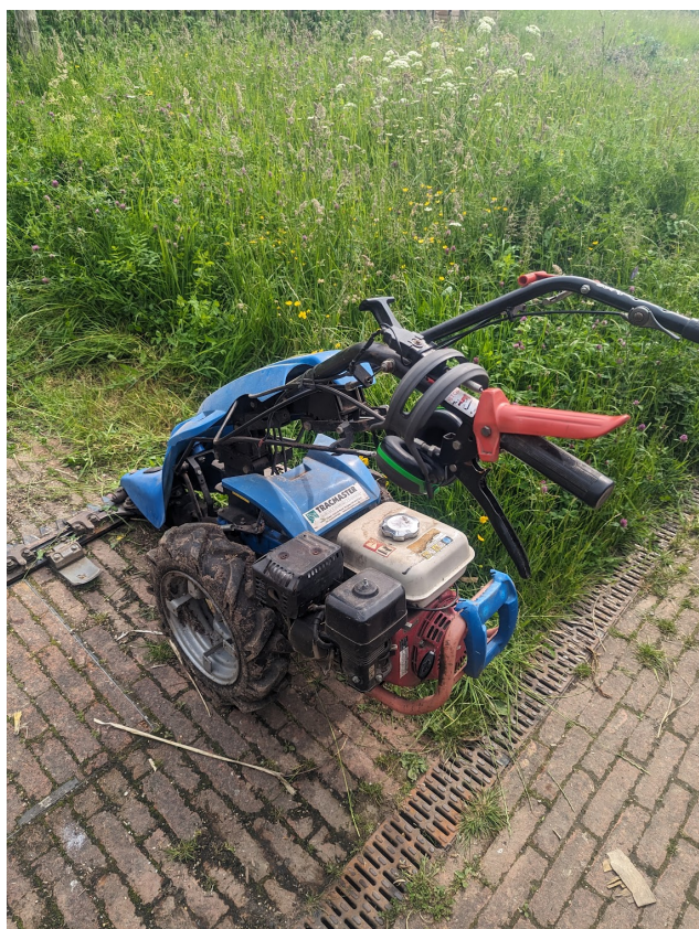
Scythe mower with petrol engine.
