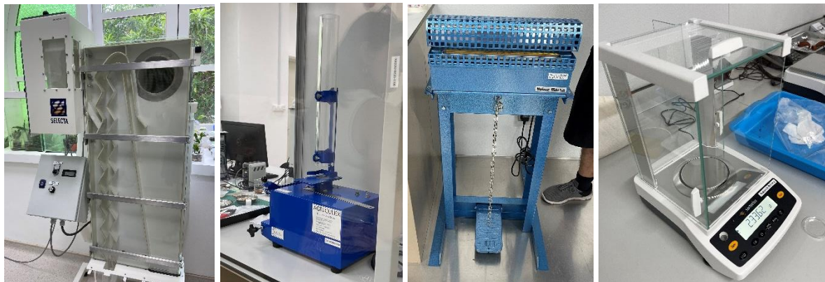
Fig.25, 26, 27 & 28. The same equipment used by SBG Seed Bank that we have at the National Seed Bank of Wales. From left to right: Selecta Zig-zag aspirator and Agriculex aspirator (used for cleaning seed), heat sealer (used for sealing foil bags before being stored in freezer), sensitive scales (used for weighing seed collections).
