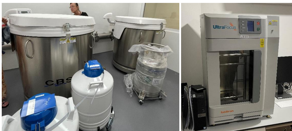
Fig.29 & 30. Left: cryogenic storage containers, for deep freezing seeds. Right: X-ray machine in dedicated room for assessing seed quality and viability.
