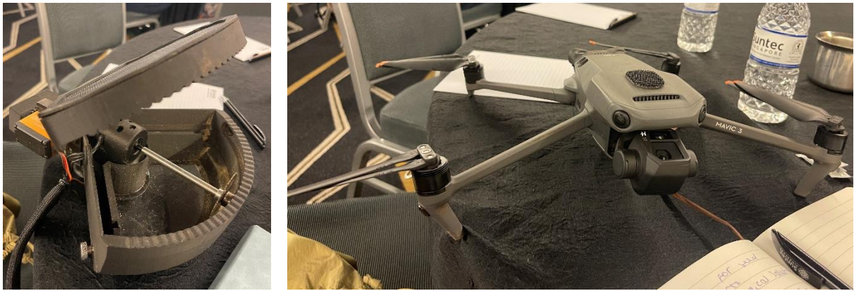
Fig.20 & 21. Drone equipment being developed to map species and collect seed from remote and inaccessible plants in Hawaii (Nyberg et al. , 2024). Left: Grabbing device attached to drone used to collect plant material and take it safely back to the researchers. Right: Drone used to map species on cliff sides.
